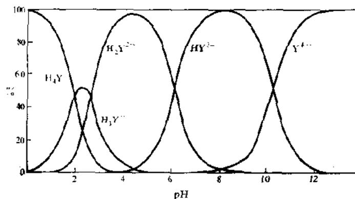
**Fig. 7** Dissociation of EDTA as a function of the pH-value [2]
