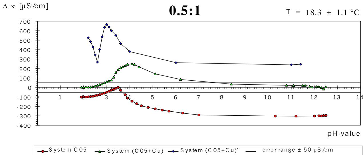
**Fig. 10** pH-spectrum of the Citr.-copper-complex System (C05+Cu), pH 4
