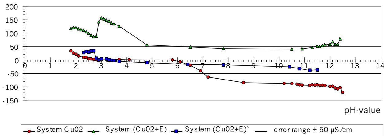
**Fig. 2** pH-spectrum of the EDTA-copper-complex System (Cu<sup>2+</sup>+E), pH 3
