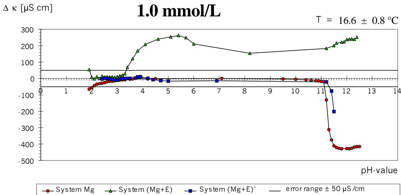
**Fig. 9** pH-spectrum of the EDTA-magnesium-complex System (Mg+E), pH 5.4
