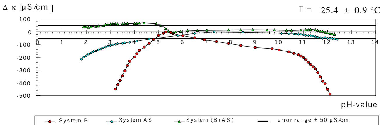
**Fig. 18** The pH-spectrum of the antigen-antibody-complex (System (B+AS), pH 4.4) between Bovine Albumin (231 mg, Fraction V Powder, Sigma Aldrich) and the antibody to Sheep whole Serum (0.3 ml, Liquid, Host Animal Rabbit, Sigma Aldrich)
