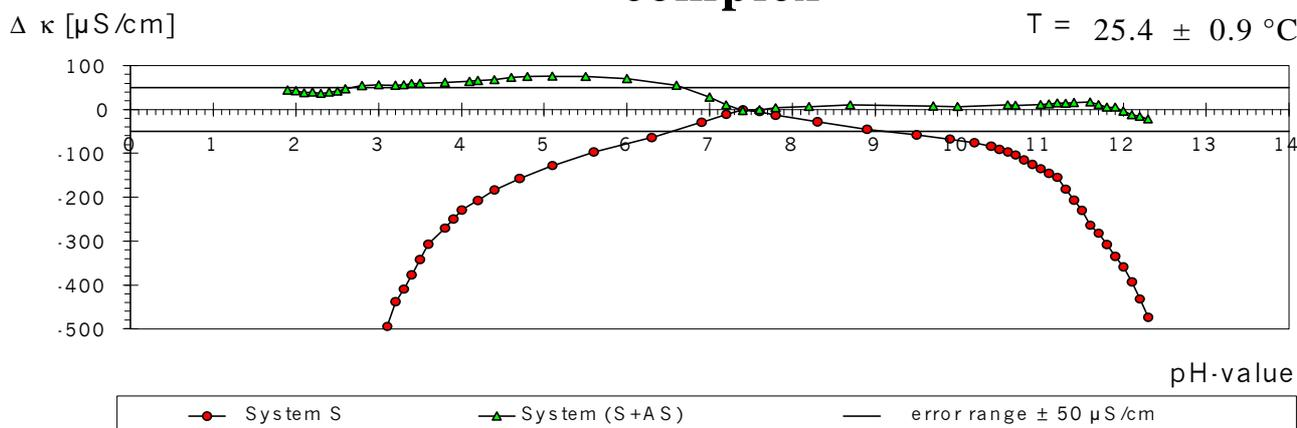
**Fig. 17** The pH-spectrum of the antigen-antibody-complex (System (S+AS), pH 5.1) between Sheep Albumin (231 mg, Fraction V Powder, Sigma Aldrich) and the antibody to Sheep whole Serum (0.3 ml, Liquid, Host Animal Rabbit, Sigma Aldrich)
