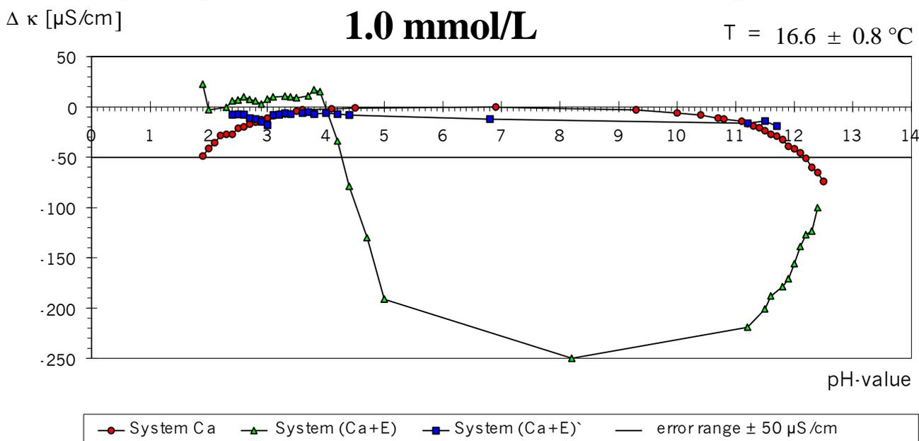
**Fig. 8** pH-spectrum of the EDTA-calcium-complex System (Ca+E), pH 8.2
