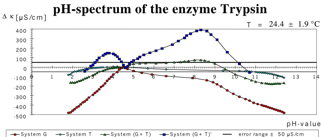
**Fig. 16** The pH-spectrum shows with the Theoprax-curve System (G+T)<sup>`</sup> the pH-activity-curve of Trypsin (20 mg Trypsin / 0.4% solution of Gelatine)
