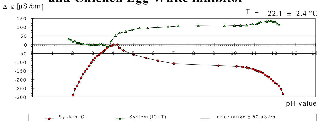
**Fig. 13** pH-spectrum of the enzyme-inhibitor-complex (System (IC+T), pH 4.3 - pH 11.8) between Trypsin (120 mg, Boehringer Mannheim, 10000 BAEE) and Chicken Egg White inhibitor (120 mg, Sigma Aldrich, 1 mg inhibit 1 mg Trypsin 10000 BAEE)
