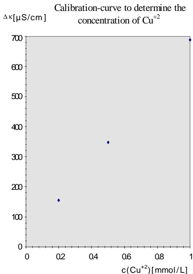
**Fig. 5** Calibration-curve to determine the concentration of  $\text{Cu}^{+2}$ , error range  $\pm 10\%$  of  $c(\text{Cu}^{+2})$  [ $\text{mmol}/\text{L}$ ]
