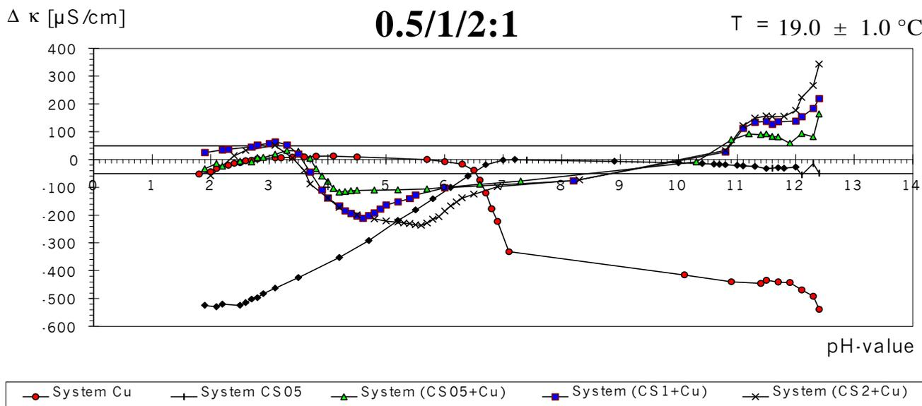
**Fig. 11** pH-spectrum of the Citr.-copper-complex System (CS05/1/2+Cu), pH 3.9/3.8/3.7 - 12.4
